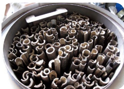
Production of bio-charcoal from bamboo.
