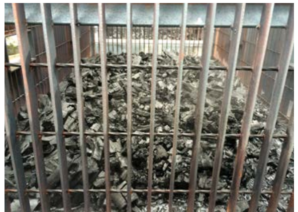
The hot biochar cooling down in the dunk tank.
