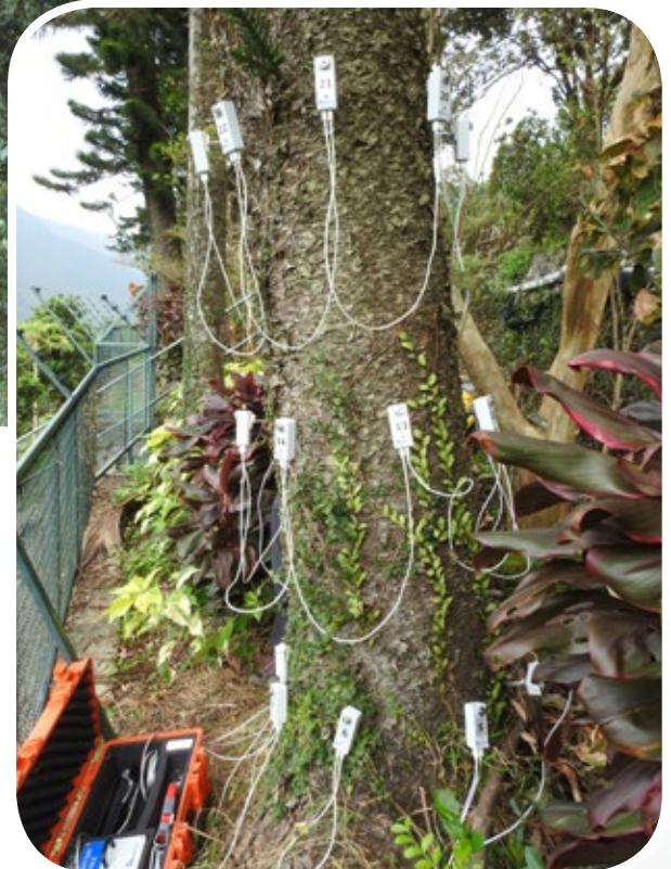
Tomograph test being conducted on an Araucaria heterophylla for checking its internal wood condition to check tree health and safety.
